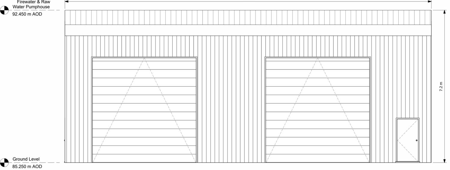
**4 Fire Water Pumphouse West Elevation**
