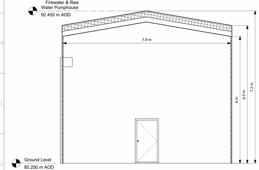
**5 Firewater Pumphouse Section A-A**
